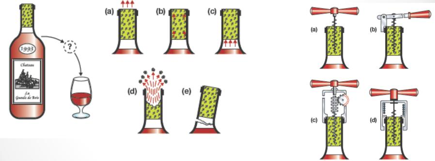
Embodiments - Sketches for devices based on axial traction The first is a direct pull; the other three use levered pull, geared pull, and spring-assisted pull
